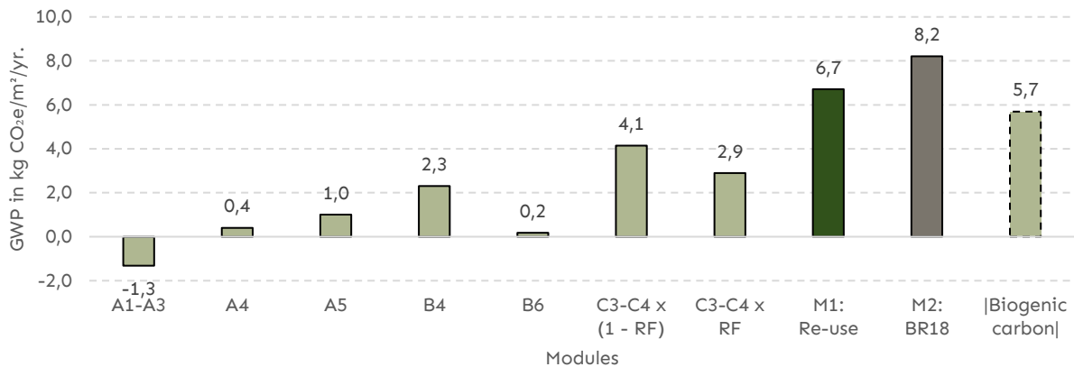
Figure 9 SFH - LCA results for lifecycle modules and LCA methods 1 and 2 for a 50-year period.
